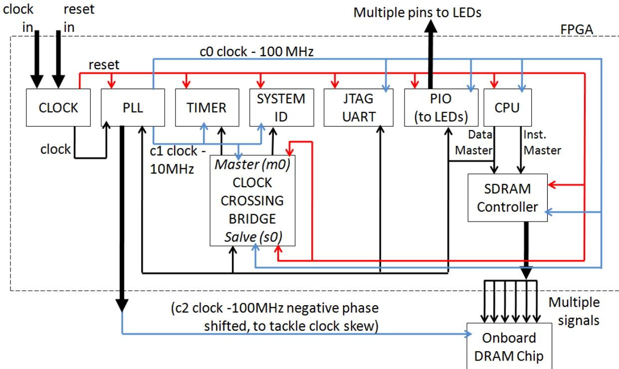
a. New hardware components to be used: *SDRAM Controller*, Avalon ALTPPLL.
