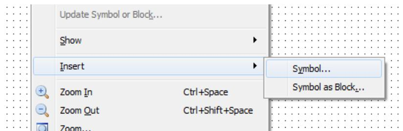
Under *Libraries->primitives->pin*, find the input pin symbol and click OK. Left-click to place the symbol on the BDF. Right click on the newly added *pin* symbol to open the Properties dialog. Rename the pin as *INPUT\_CLOCK*.
