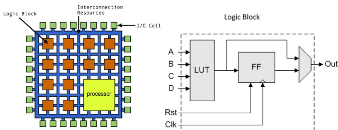
Each logic block can be configured to implement different logic functions. By combining many such blocks and customizing their interconnections, one can construct very sophisticated circuits, including complete computer processors. A processor designed, synthesized, and mapped onto these logic blocks can then execute software programs just like a processor built as a traditional integrated circuit.
