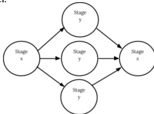
This approach increases hardware resource usage but can significantly improve performance when the workload is highly parallelizable.
